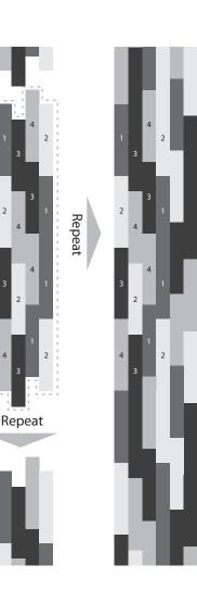
Based on TOP line, 4 planks in a row are laid 4 times in a fixed order and a set of 16 planks is repeated to cover the expanded space.
