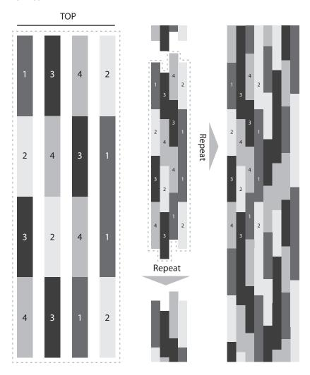
Based on TOP line, 4 planks in a row are laid 4 times in a fixed order and a set of 16 planks is repeated to cover the expanded space.
